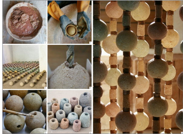
Figure 5. The process of making Sarooj Balls and installing the shader in the Ultrasound Room.
